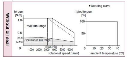
Dotted line represents the torque at 10 % less supply voltage.
